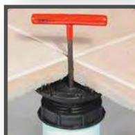
**Self-Leveling** head allows for slope compensation of 0% to 4% in any direction. Allen or Hex key will allow for leveling while loaded with pavers. *Eliminates having to remove pavers to make adjustments!*
